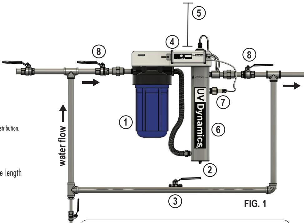
**UV Dynamics Mini-Rack Systems feature a 'U' shaped bracket that enables you to install the system in either direction to accommodate both L-R and R-L water flow!**
